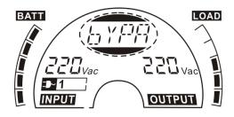
Figure 6.3 The Bypass mode
