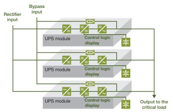
In DPA, each UPS module has all the hardware and software it needs for autonomous operation.
